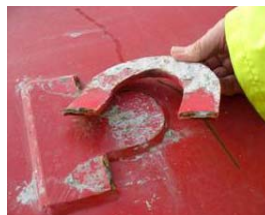
Incident 2 involved an empty 1000 litre roll-over concrete skip, slung horizontally by the lifting point
