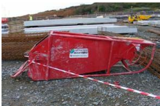
Incident 2 involved an empty 1000 litre roll-over concrete skip, slung horizontally by the lifting point
