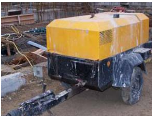
Incident 1 involved a wheeled compressor slung by the single lifting point
