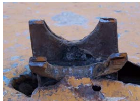
Incident 1 involved a wheeled compressor slung by the single lifting point
