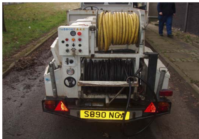
High Pressure Mobile Jetting Unit similar to the one involved in the incident
