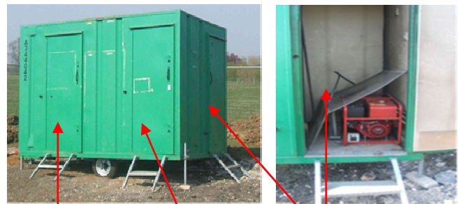
Mess Room Toilet Generator Room
